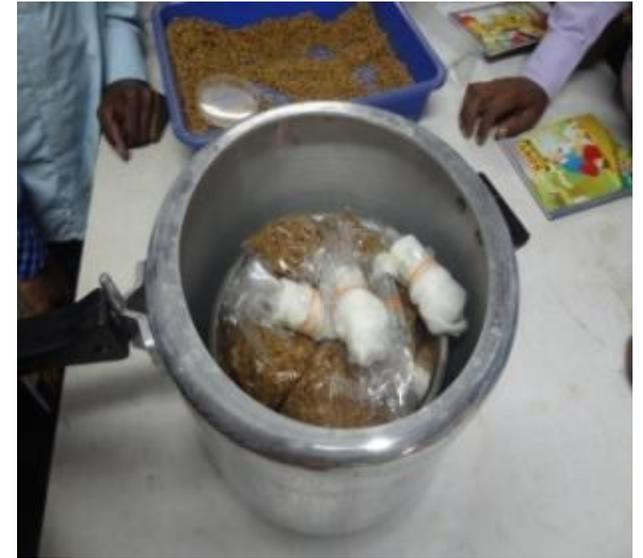
Put the poly bags of grains inside the pressure cooker and boil for 20 min at low heat (minimize the flame after 1<sup>st</sup> whistle)
